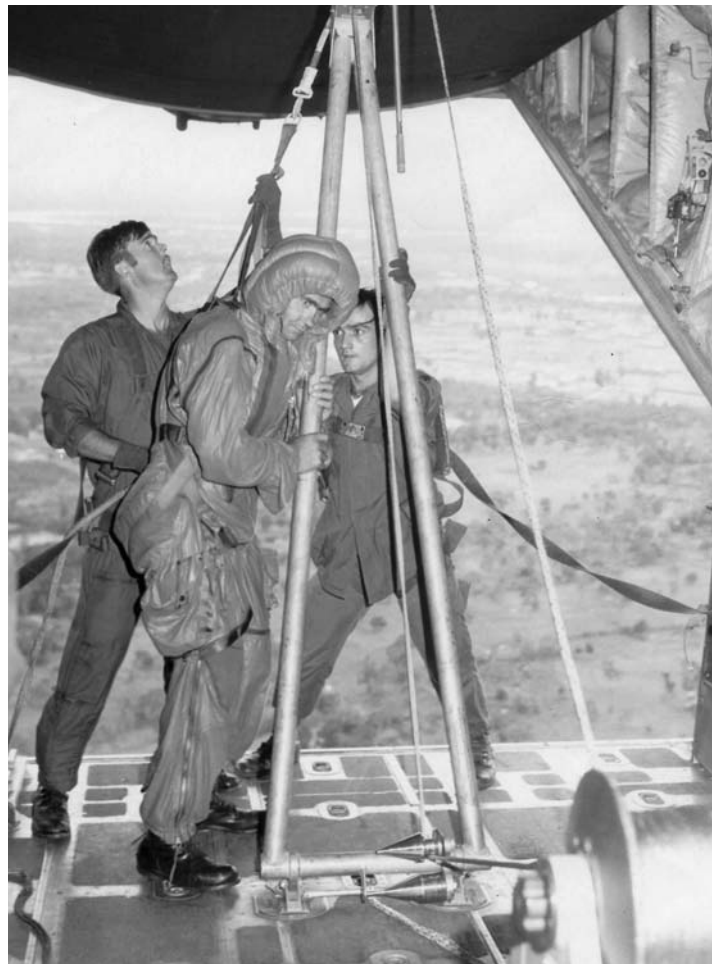
A successful use Fulton Skyhook Aerial Retrieval System in Thailand, Oct. 31, 1970. Courtesy photo.
