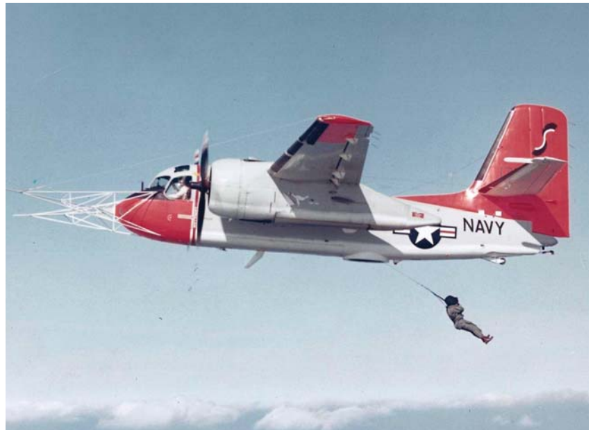
A U.S. Navy S2 tracker testing the Fulton Skyhook Aerial Retrieval System. Courtesy photo.
